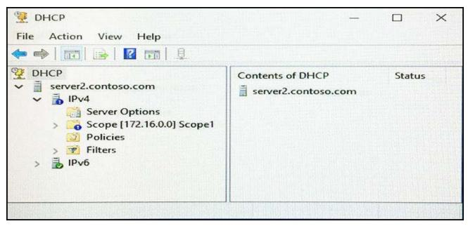
Scope1 has an address range of 172.16.0.10 to 172.16.0.100 and a prefix length of 23 bits.
