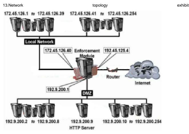
You want hide all localnet and DMZ hosts behind the Enforcemenet Module, except for the HTTP Server (192.9.200.9). The HTTP Server will be providing public services, and must be accessible from the Internet.
