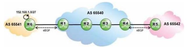
AS 65540 is using MPLS to provide BGP shortcuts for its iBGP routing.
