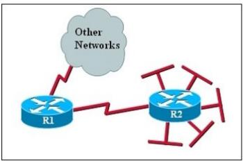
The networks connected to router R2 have been summarized as a 192.168.176.0/21 route and sent to R1.
