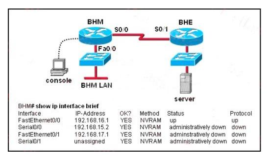
Users on the BHM LAN are unable to access the server attached to the BHE router.
