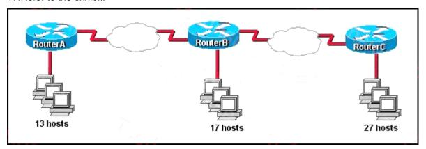
The internetwork is using subnets of the address 192.168.1.0 with a subnet mask of 255.255.255.224.
