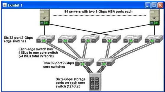
You are designing a new SAN. The existing SAN uses eight 32-port 2-Gbps Fibre Channel switches. Two of the switches are deployed as core switches, and the remaining six switches are deployed as edge
