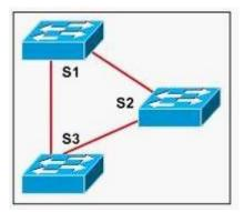
A.IEEE 802.1w, and IEEE 802.1s are compatible. IEEE 802.1d is incompatible. Switches S1 and S3 will be able to pass traffic between themselves. Neither will be able to pass traffic to Switch S2.
