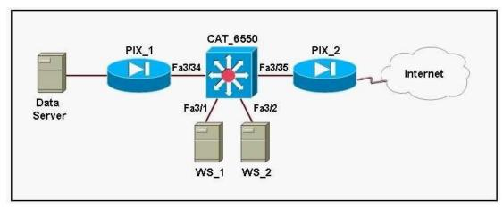
A.The switch ports 3/1 and 3/2 will be defined as secondary VLAN isolated ports. The ports connecting to the two firewalls will be defined as primary VLAN promiscuous ports.
