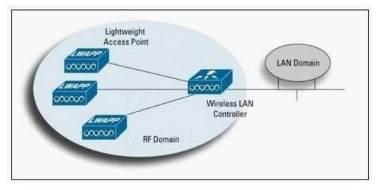
A.An AP that has been upgraded from an autonomous AP to lightweight AP will only function in conjunction with a Cisco Wireless LAN controller.
