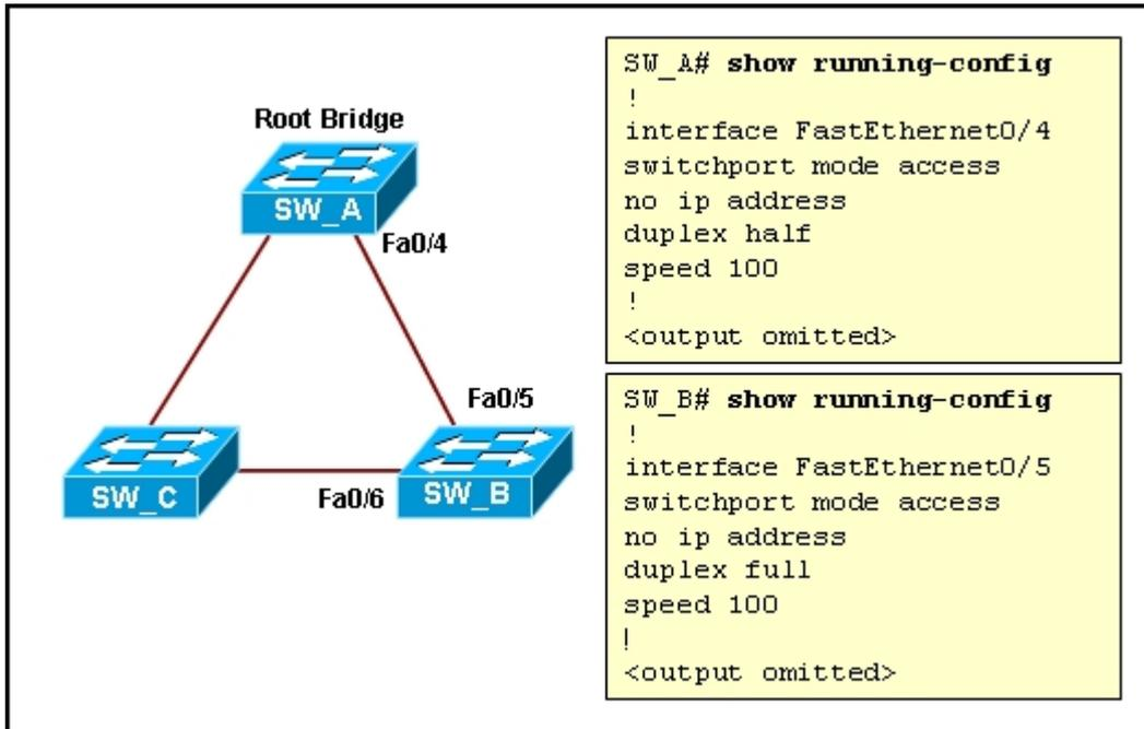
and the partial configuration of switch SW\_A and SW\_B. STP is configured on all switches in the network. SW\_B receives this error message on the console port:
