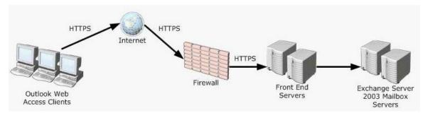
Server 2003 messaging system. Your company has two Exchange Server 2003 front-end servers deployed in a Network Load Balancing cluster, as shown in the following diagram:
