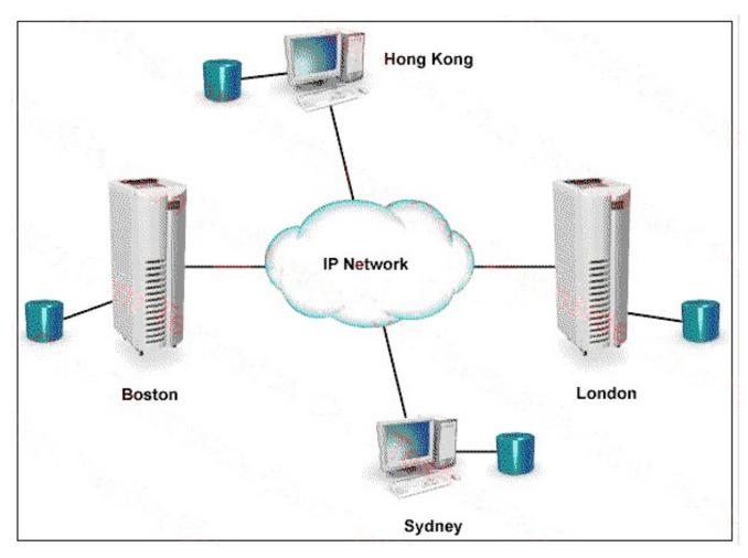
Two Celerras are located in London and Boston. A NAS solution is required that maintains a copy of the
