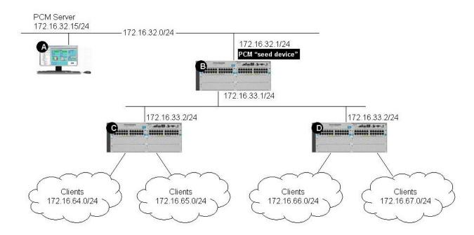
You have installed PCM+ and all of its plug-in applications on the network shown in the exhibit. You have not performed any additional configuration. Which device(s) will be included in the network map when you log in to PCM+ for the first time?
