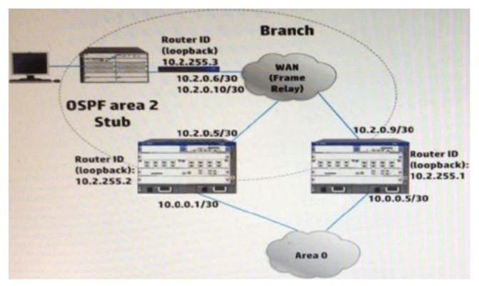
The branch routers have E1 lines into the Frame Relay service provider network. The exhibit shows just one branch but the network actually has 30 branches. The Hp 6600 Services routers, which are the area border routers (ABRs), have E3 lines into the Frame Relay network. The routers in the exhibit implement Open Shortest Path First (OSPF).
