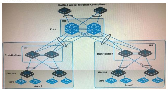
A company has HP APs that are managed by the two Unified Wired-Wireless controllers. Wireless users use Wi-Fi Protected access (WPA2) and authenticate with 802.1X to HP Access Manager (UAM). The SSID uses centralized forwarding. Users need to be able to roam seamlessly from area 1 to area 2. Which step helps to meet these needs?
