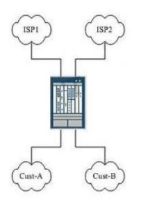
In the exhibit, Customer A and Customer B connect to the same SRX Series device. ISP1 and ISP2 are also directly connected to the SRX device. Customer A's traffic must use ISP1, and Customer B's traffic must use ISP2.
