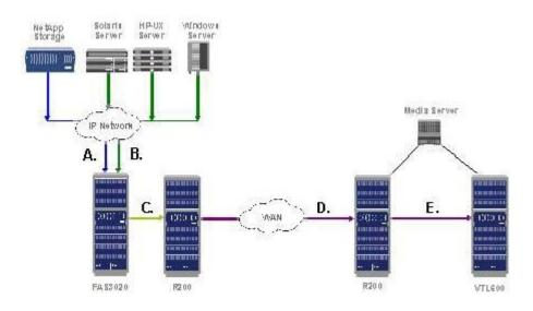
A. (A) SnapVault, (B) OSSV. (C) SnapVault, (D) Async SnapMirror, (E) NDMP
